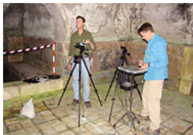
GCI scientist using laser speckle interferometry to detect areas of detachment in wall paintings at the site of Herculaneum. Photo: Giacomo Chiari
