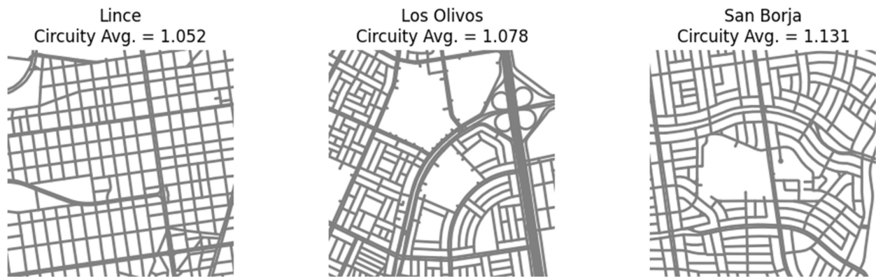
Figure 2. Examples of urban grids in three districts of Lima (Lince, Los Olivos, and San Borja) at 1 square kilometre. Lince was urbanized in the early twentieth century, while Los Olivos and San Borja between the 1960s and 1980s. The plots are organized left to right by levels of circuitry average. I explain this variable in Section 2; in sum, it indicates the sinuosity of the street layouts. Part of my argument below is that more sinuous layouts (e.g., San Borja) facilitate the construction of micro-segregating infrastructure.
